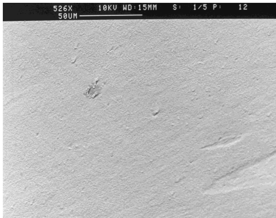
Figure 12 Surface fracture observation of 50PVC/50PU1/5 blend ( \times 526 ).
